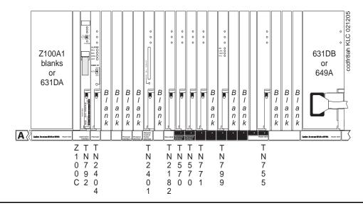
The control carrier has dedicated white-colored circuit pack slots that always contain specific control circuit packs. Dual-colored slots can contain any port circuit pack or the designated white circuit pack, such as a DS1 circuit pack or a power unit. AC or DC input power supplies provide power to the carrier.
