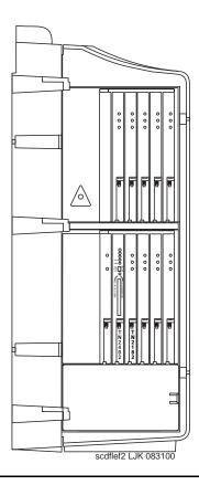
The following figure shows the connections on the right side of the cabinet of the CMC1 Media Gateway. From 1 to 10 25-pair connectors provide an interface between port circuit packs and the cross-connect field or a cable access panel.
