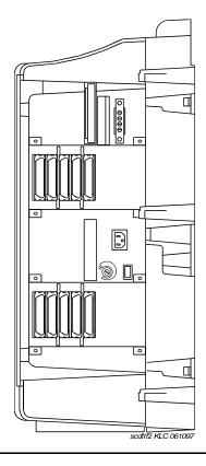
The following figure shows a front view of a cabinet containing three CMC1 Media Gateways.
