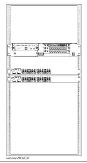
Figure 45: G700 Media Gateway with two Avaya C360 switches
