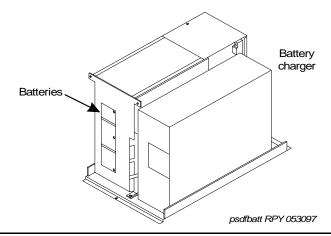
The battery charger is used only without an uninterruptible power supply (UPS). The charger contains:
