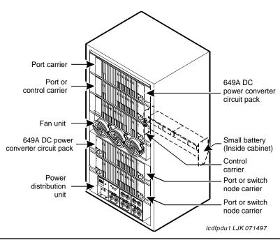
The following figure shows the DC power distribution in some MCC1s with large batteries or extended battery backup. Switch node (SN) carriers require two 649A DC power converters and two cables.
